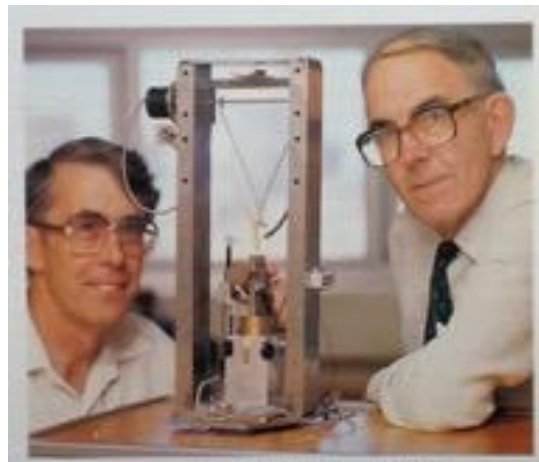
The writer (left) (and his plant-breeder colleague) with the mechanical instrument which the former designed to measure shatter resistance of canola pods under impact.
